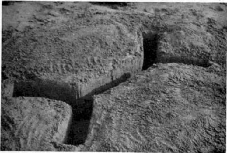
Photo 8. A 1 : 6 scale model in sand of the excavation required for a typical Battle Shelter for four men.
