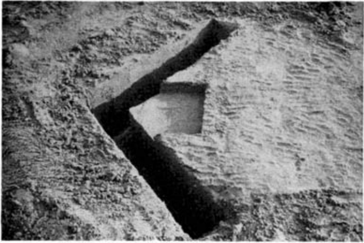
Photo 7. A 1 : 6 scale model in sand of the excavation required for a medium machine gun Battle Shelter.
