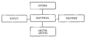
Input may employ punched paper tape, which is prepared by the use of a special teleprinter.
