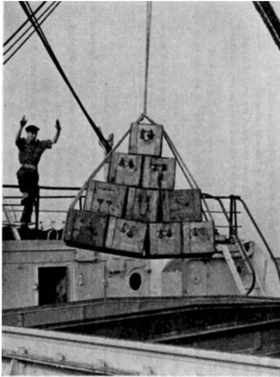
Photo 1. Hatchwayman signalling a load of boxes into the hold.
