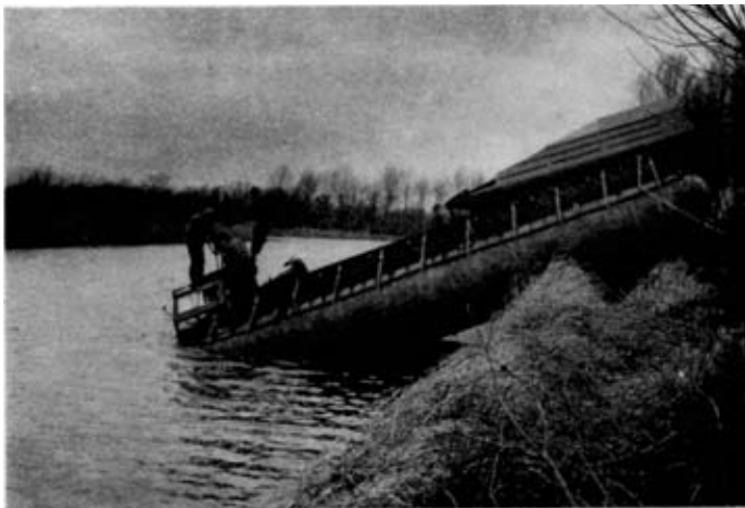
Photo 5. —The Amphibious ferry being launched over a 5-ft. bank.
