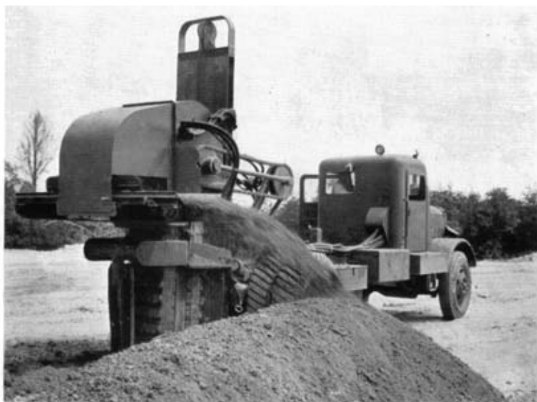
Photo 6. —A trench digger that can dig a fox hole in ten seconds.
