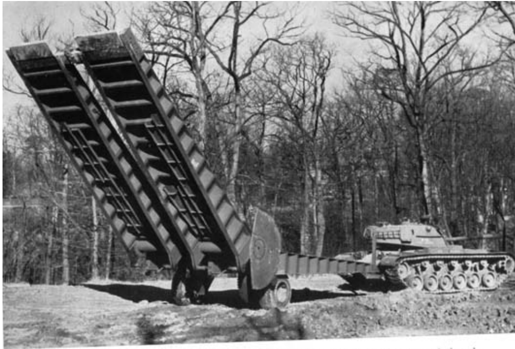
Photo 1. —A short span bridge capable of carrying tanks, which can be put in position by an operator in the tank.
