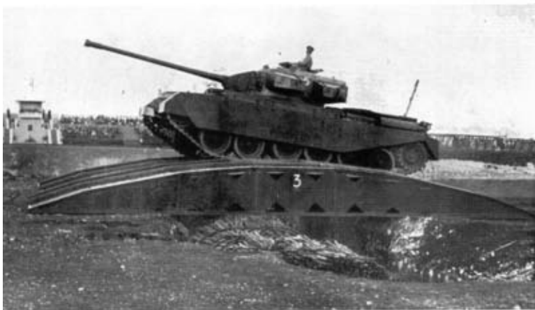
Photo 9. —A Centurion tank crossing a tank bridge previously laid by a special Bridge-laying tank.
