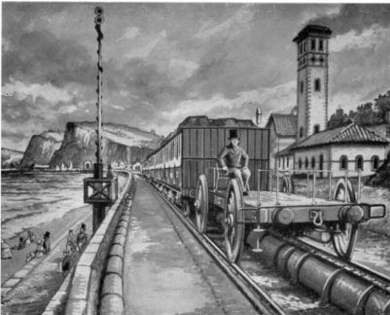
Photo 2. —Atmospheric system on South Devon Railway.
