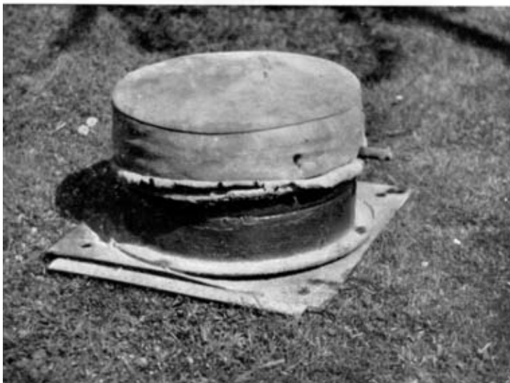
Photo 2. —B Type C mine complete as frequently found to-day. Note arming handle and rubber cover.
