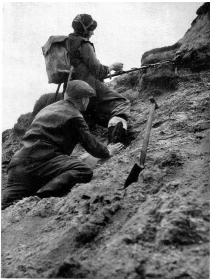
Photo 3. —Using a No. 4A detector on soft cliff. Note how one man assists the other. (Photo : Eastern Daily Press. Norwich )
