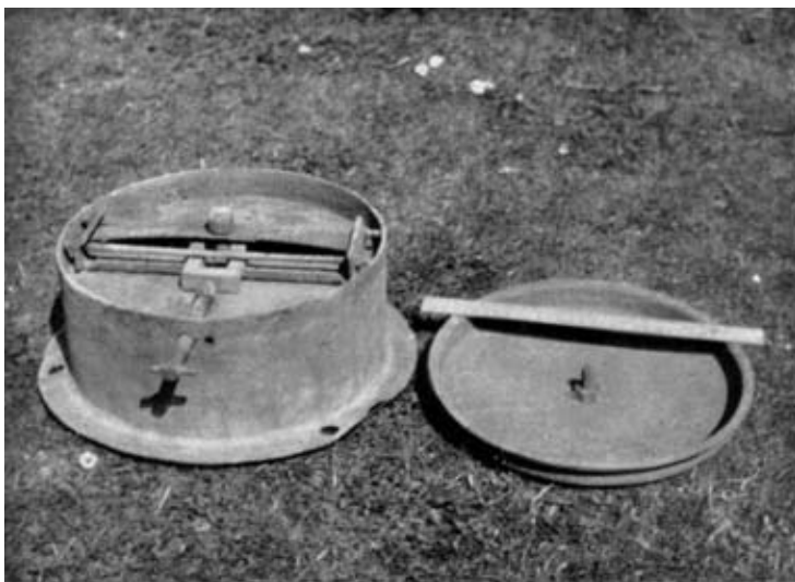
Photo 1. —B Type C mine with rubber cover and lid removed.
