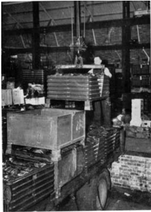
Photo 1. —Box pallets being unloaded by crane.
