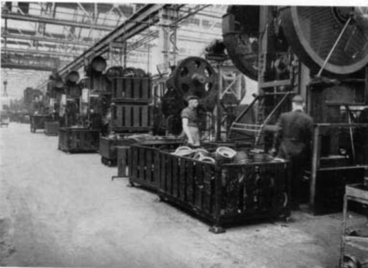
Photo 4. —Box pallets being used in a flow sequence for material going through a press shop. Note space saving in the background where box pallets have been stacked three high.
