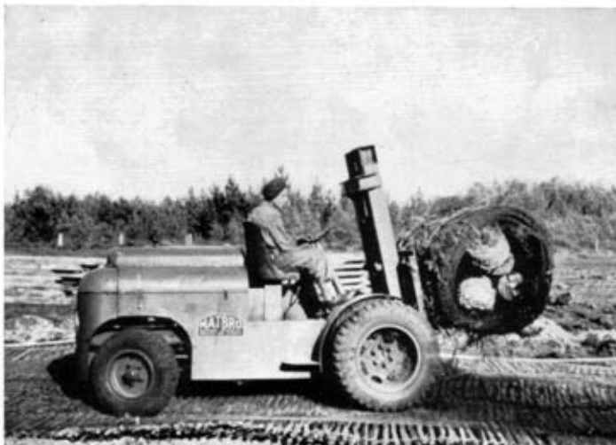
Fig. 4.—2-ton "Matbro" forklift truck carrying barbed wire parcel along a temporary track.
