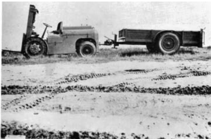
Fig. 1. —Mathew Brothers' 2-ton "Mathbro" forklift truck towing 3-ton Tasker trailer. Note the built-in stabilizing jacks on the trailer. The front and tail boards are removable, and can be used as ramps.
