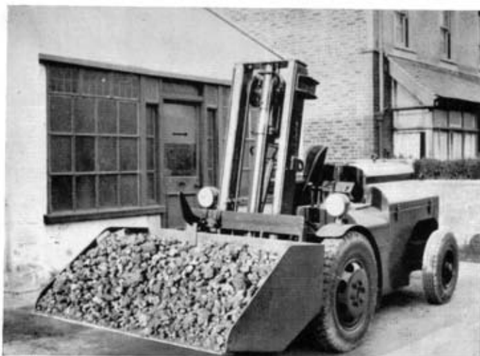
Fig. 2. —2-ton "Mathbro" forklift truck fitted with 1-cu. yd. shovel in lieu of forks.
