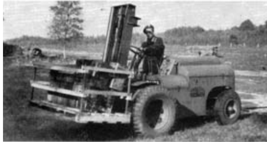
Fig. 5. —2-ton "Matbro" forklift truck carrying a field-made 6 x 3 ft. 1 ton capacity, tray pallet with removable rail sides. The pallet is loaded with ammunition boxes filled with nails as part of the engineer stores in the Corps Maintenance area for Exercise "Surprise Packet".
