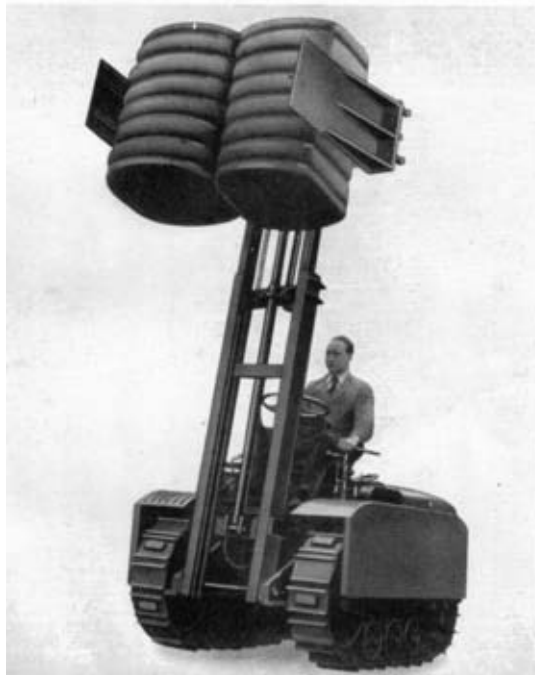
Fig. 6. —Stockport Manufacturing Company's 1,000 lb. capacity prototype-tracked forklift truck "Roughrider", with "The Rodman" hydraulic clamp device, holding two cotton bales.
