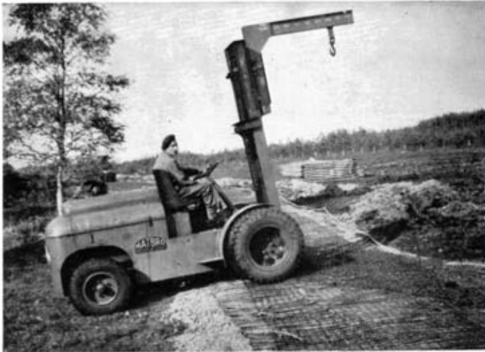
Fig. 3.—2-ton "Matbro" forklift truck fitted with crane jib in place of forks.
