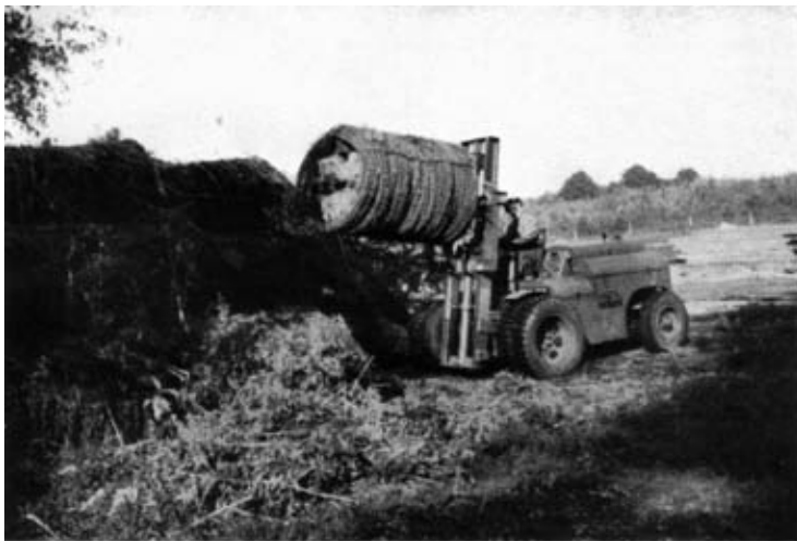
Fig. 5.—"Matbro" cross-country forklift truck handling parcelled barbed wire in C.M.A. for Exercise "Surprise Packet." The truck has been fitted with its jib arm in place of the forks.
