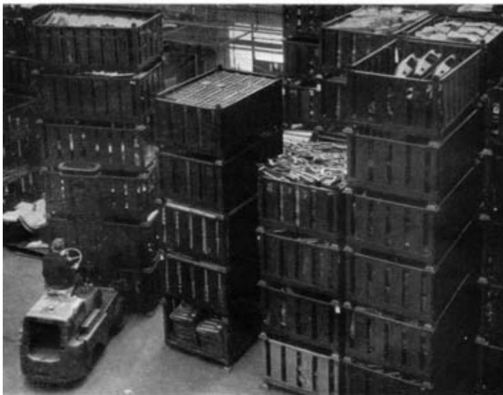
Fig. 6.—6 × 4 ft. box pallets being used for local palletization in Messrs. Fisher and Ladlows' works.
