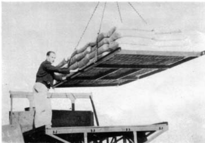
Fig. 8.—12 × 6 ft. pallet/cargo board loaded with 3 tons of hydro lime.
