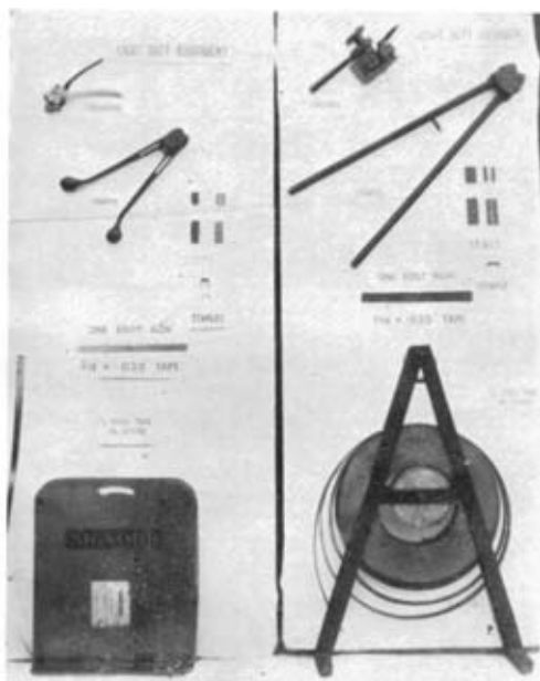
Fig. 1.—Light and heavy duty steel tape and tools and equipment for applying it.
