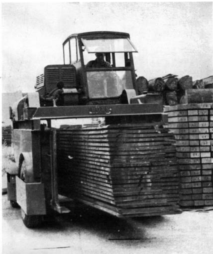
Photo 1. —ROSS, SERIES "70" STRADDLETRUCK. Picking up the load.—Note "Stool" is under the load and the height of the load permits locking against underside of carriage for rigid transport.
