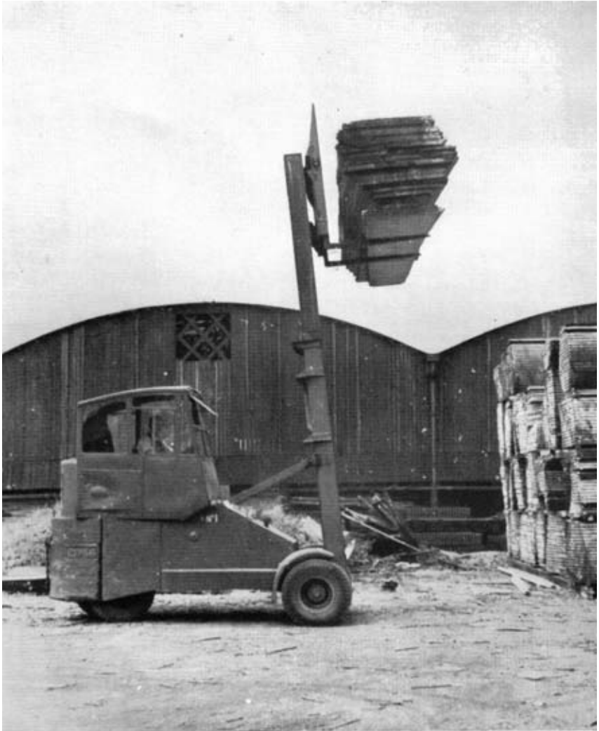
Photo 2.—Ross (5-TON, 22 FT. LIFT) FORK TRUCK. Side view of load at maximum elevation.
