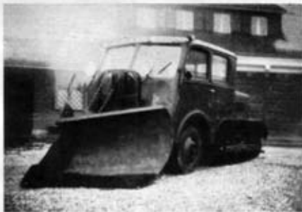
Photo 3. —A.F.R. half-track vehicle fitted with Grassmuck plough.
