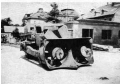
Photo 4. —"Schleuder" plough with rotors, fitted to Ost.
