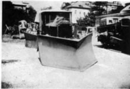
Photo 2. —Daimler-Benz truck fitted with front and side ploughs.
