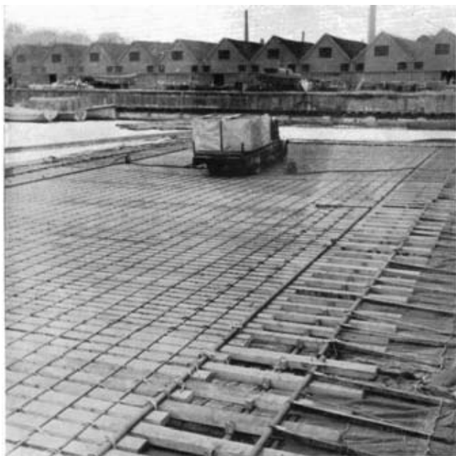
Photo 4.—"Clover" Mk. I, Static load test.
