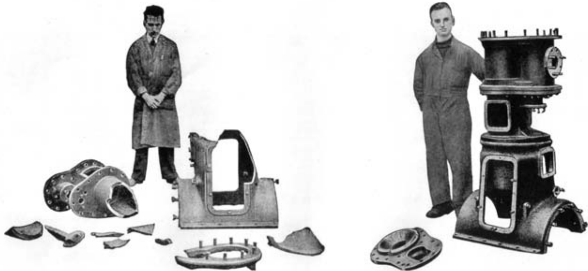
Plate 6.—Badly damaged steam engine ; repaired steam engine.
