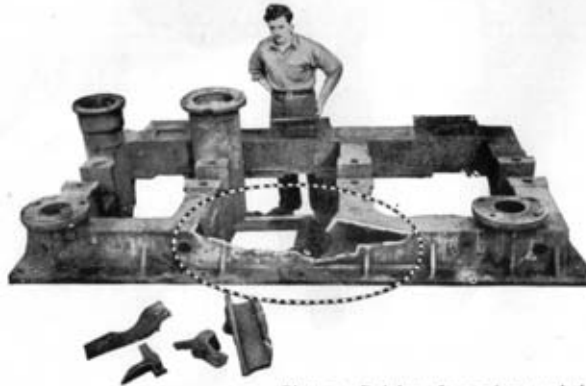
Plate 5.—Bedplate of sea-going vessel, damaged by enemy action ; bedplate after repair.
