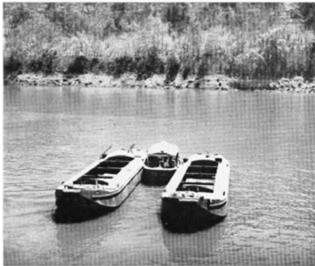
Photo. 2.—Typical tow. Single screw Unicraft Tug and two Barges.
