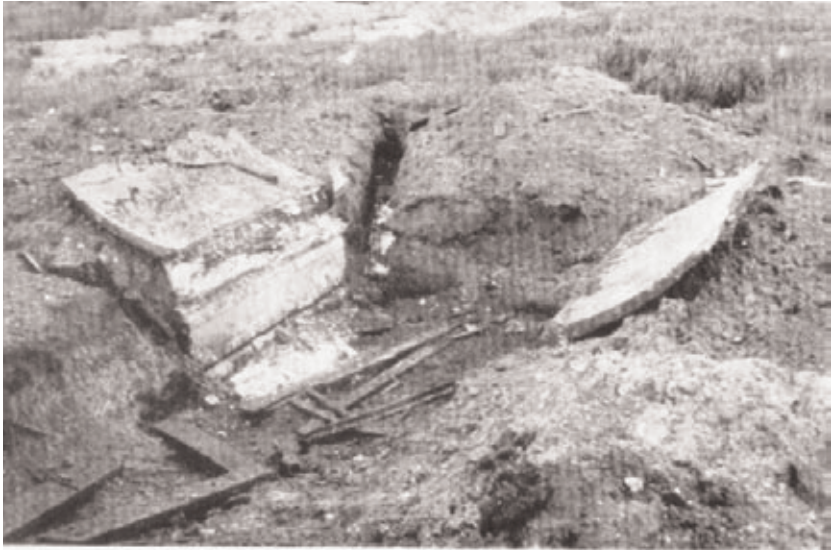
Fig. 1.—Demolition test on 1/10th-scale model of vault arch bridge. (Note two halves of arch folded back.)
