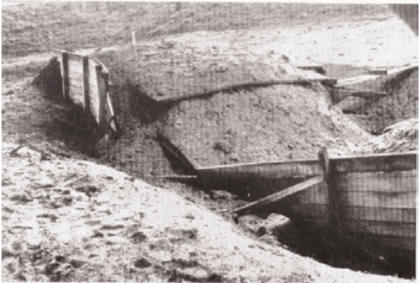
Fig. 2.—Demolition test on 1/4-scale model of vault arch bridge. (Note two halves of arch collapsed between abutments.)
