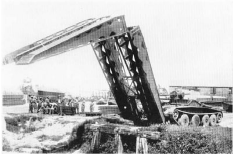
Plate 3.—30 ft. Scissors Bridge, carried on Covenantan Bridgelay, being launched.
