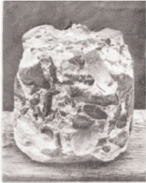
Fig. 1.—Core cut from Concrete Road grouted with Colloidal Grout, showing the completeness with which the Colloidal Grout penetrates the aggregate.
