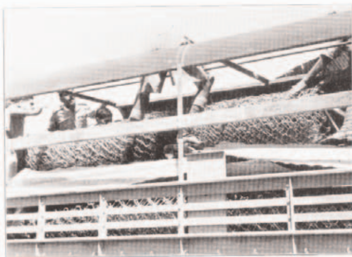
Nearly a lorry-load. Roofing-iron is being used to keep the rolls apart, and the roof cover has been removed from the lorry.
