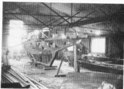
2.—(Dec., 1937.) The moulds up and the beam shelves in position.
