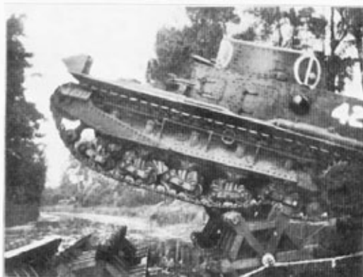
2.—Medium tank on second stone, just about to drop on to third stone. This is considered about the maximum amount of drop advisable when a large number of tanks have to cross.
