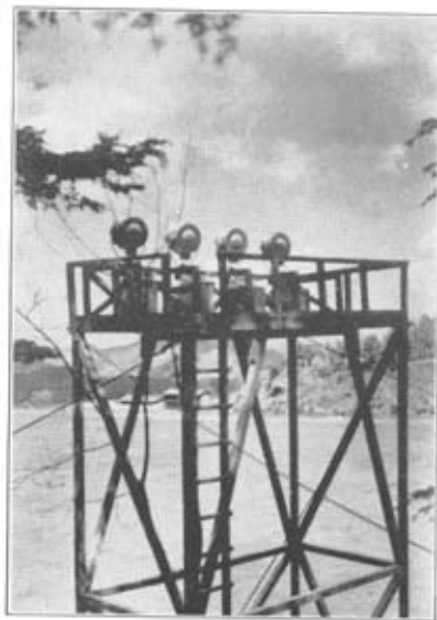
Photo No. 2.—Tower arrangement. Each light can traverse 90° right to left without interference with others.
