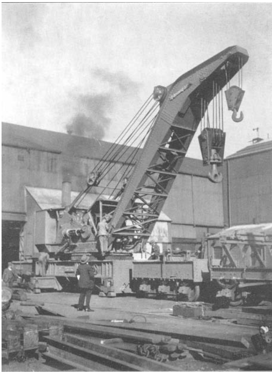
No. 1.—Crane in working order, showing props.
