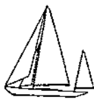
DORADE , 21 tons Owner: Messrs R. & J. Scammell (U.S.A.) Built in 1930 Length (overall) 52.2' Beam 10.3' Draught 7.5'
