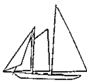
GRENADIER , 39 tons Owner: Messrs H.R. & S. Morris (U.S.A.) Built in 1930. Length (overall) 59.4' Beam 13.8' Draught 11.2'
