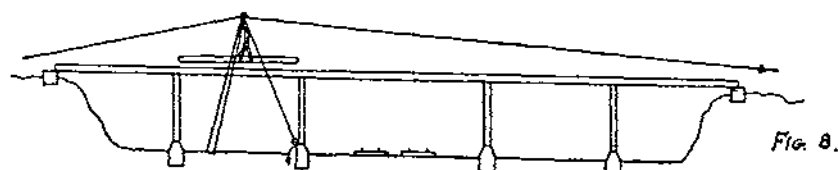
LOWERING LAST GIRDER INTO POSITION
