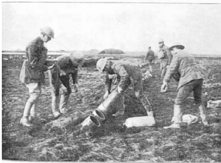
Photo II.—Livens Projectors being Loaded.
