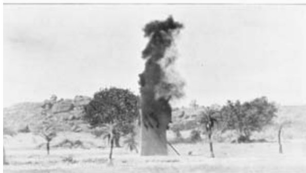
No. 2.—Failure No. 1; wet guncotton dated "1886." Dense red fumes of \text{NO}_2 evolved.
