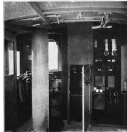
L. & S. C. R.—Interior of Sward's Compartment, showing Motor-mount Compartment and High Tension Switching Space.
