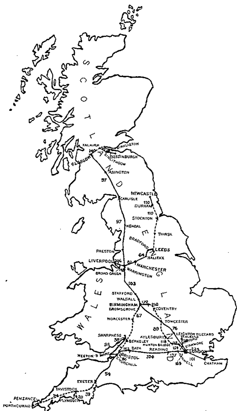
MAP 1.— The System of Underground Telegraphs either existing or under construction in the British Isles in 1908.
