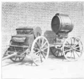
New Limber and Trail Carriage, carrying a 90-cm. Projector. Weight behind team, 32 cwt.
