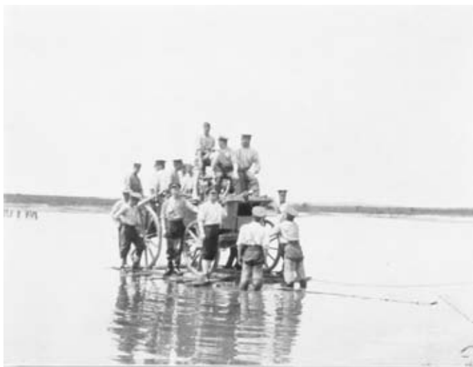
1. G.S. Wagon on Raft made of Waterproof Bags.
