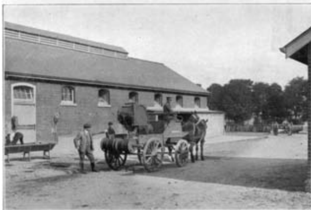
24 inch Projector on 14 cwt. R.C.D. Wagon, with cable on special axle in rear.
