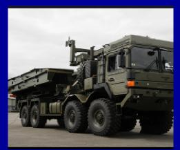
support MLC (Military Load Class) 40 wheeled and tracked vehicles under normal crossing conditions. It can also support up to MLC 50 wheeled vehicles under a caution crossing.
