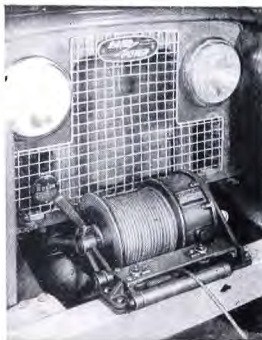
2,500 lb. Horizontal Winch front Mounted on Land Rover
