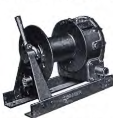
2,500 lb. Horizontal Winch. Rope Drum Barrel dia. 4". Rope Drum capacity 150 ft. \frac{3}{16} " dia. Separate Clutch is provided on the Rope Drum for easy pulling out of Winch Rope
