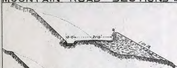
Fig. 1 for slopes from level to 1 in 2 in soft soil
